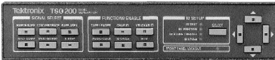
Figure 4-2. The Tektronix TSG 200 provide multiple black burst signal outputs for economically genlocking small studios. Additional features on the TSG 200 can be used for basic video testing and other odd jobs around the studio, including ID generation, setting up picture monitors and blanking tapes.
