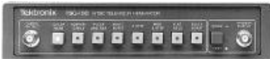
Figure 2-1. The Tektronix TSG 100 NTSC Television Generator produces a variety of special signals for testing video equipment and systems. (NTSC stands for National Television Systems Committee, the committee that developed the television system we use in the United States.)
