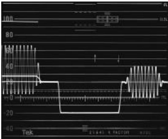
Figure 4-4. Waveform monitor display of the reference sync pulse edge adjusted to correspond to a major timing mark. This timing mark can now serve as the zero reference for individually adjusting the H-phase of each piece of video equipment in the system.
