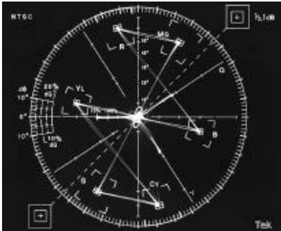
Figure 3-1a. The vectorscope screen shows a display of a SMPTE color bars test signal with all of the dots in their boxes and the color burst correctly placed on the horizontal axis.
