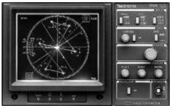
Figure 2-3. The Tektronix 1720 Vectorscope complements a waveform monitor by providing additional information about the video signal's color (chrominance) content.
