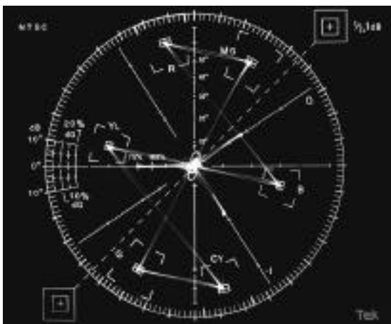
Figure 4-5. Vectorscope display of the reference color burst vector adjusted to the 9 o'clock position. All other pieces of equipment should be SC-phase adjusted to correspond to the 9 o'clock reference.
