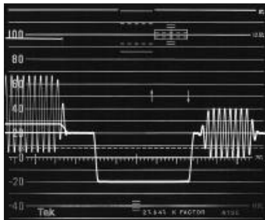
Figure 2-12. Sync pulse display horizontally magnified (MAG) and positioned vertically so the pulse's 50% levels are on the 0 IRE horizontal axis.
