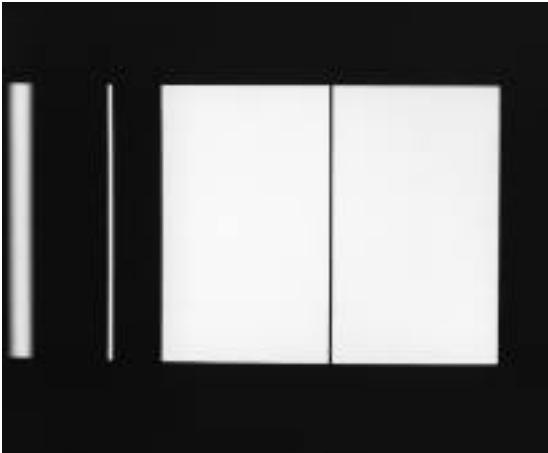
Figure 5-7. The windowed pulse and bar signal is used to check for low-frequency distortions at the field rate.
