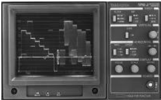
Figure 2-2. The Tektronix 1710J NTSC Waveform Monitor displays video signals for amplitude and timing measurements.
