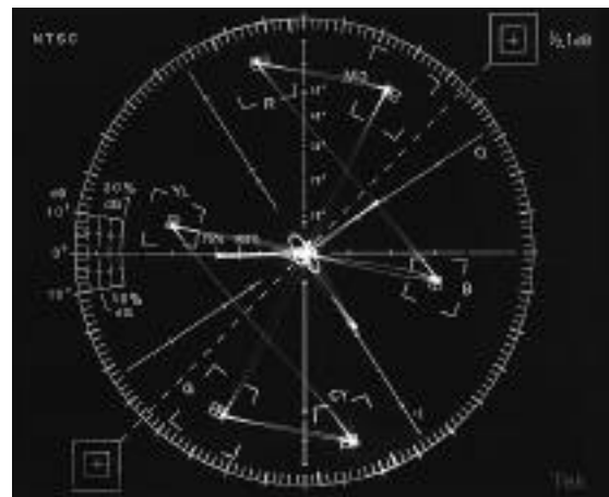
Figure 5-5. A vectorscope display of a SMPTE color bars test signal. All of the dots should be in their boxes when the color burst is aligned with the horizontal axis.
